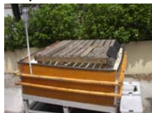
Figure 1: Deck used to evaluate leachable metals
