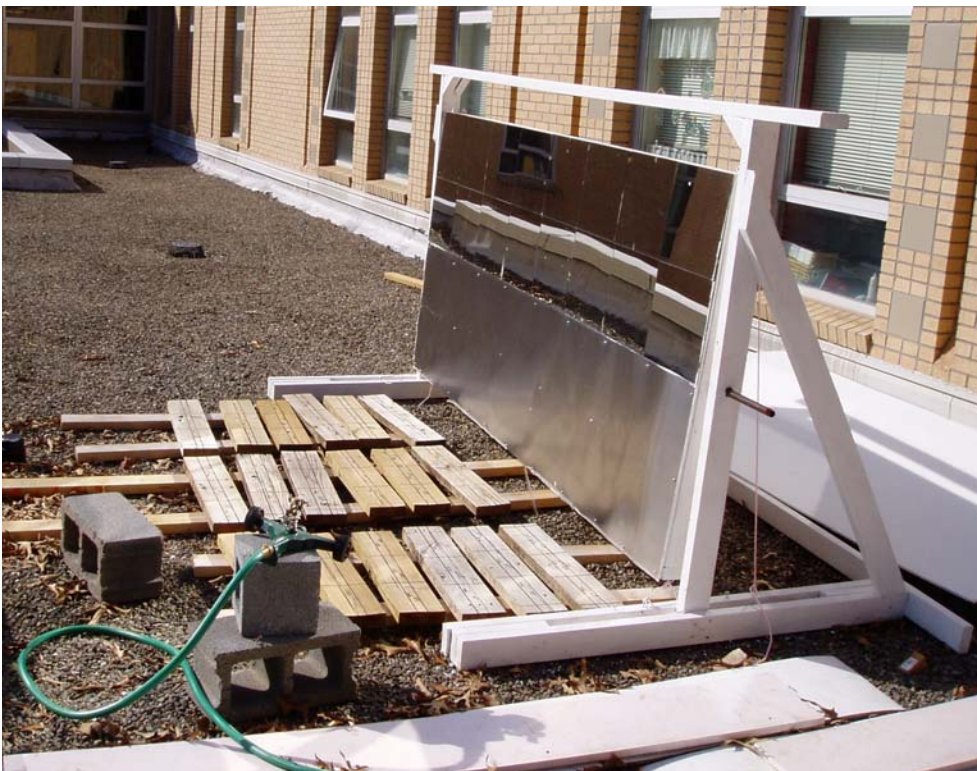
Figure 4 Photograph of accelerated aging experimental set-up with reflectors and sprinkler.
