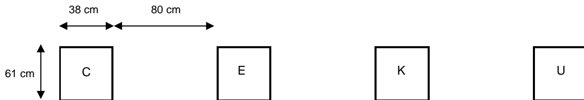
Figure 1: Layout of treatments. C = CCA; E = Copper Azole; K = kwila; U = rainwater only, from the X (unpopulated) deck; O = unwatered “dry” controls between each area.
