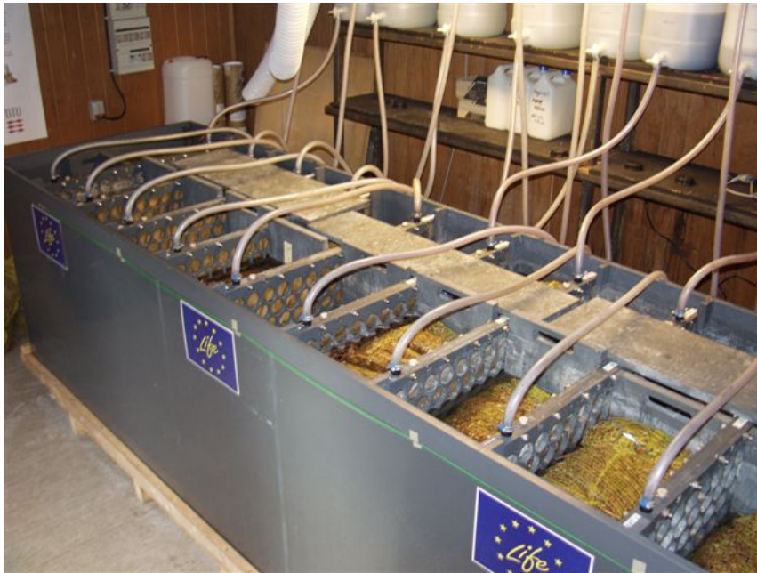
Figure 3 The pilot plant in use. Wood chips in yellow plastic nets are placed between collecting units, where the Cu, Cr and As from the wood is collected. The end units contains the electrodes, and are named electrode units.
