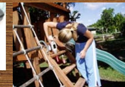
Figure 11: Analyzing a playground using an XRF unit
