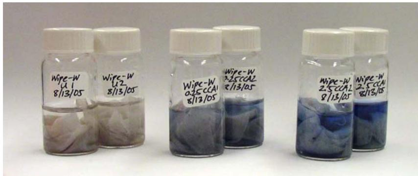
Figure II.9: Picture of Wipe Samples from Weathered Untreated,  $4.0 \text{ kg/m}^3$  CCA, and  $40 \text{ kg/m}^3$  CCA-Treated Wood with the Stannous Chloride Stain
