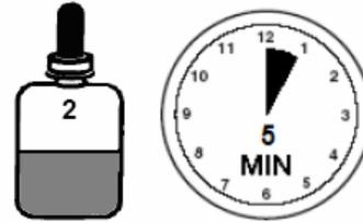
5. After 5 minutes, remove the reaction vessel cap and add 9 drops of Reagent 2 into the reaction vessel.
