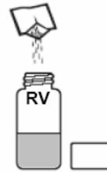
7. Replace reaction vessel cap, shake reaction vessel to mix, and let stand. Allow reaction to occur for 45 minutes.
