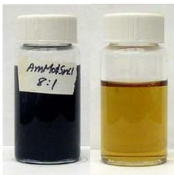
Figure II.7: Picture of Modified Stannous Chloride Stain (left) and Diluted Stannous Chloride Stain (right)
